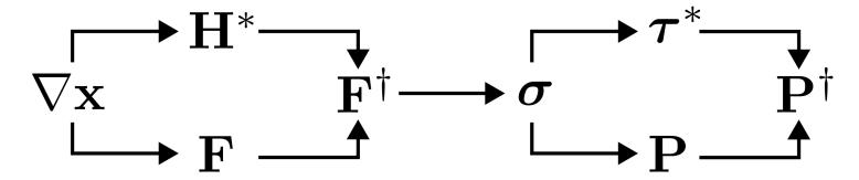
• Element internal forces integrated using the modified first P-K stress:
